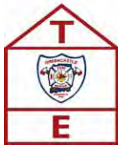
FIGURE 316.6.2 EXAMPLE STRUCTURAL IDENTIFICATION LABEL
